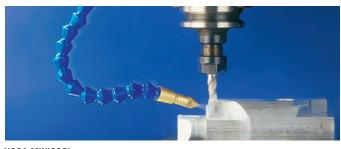
**NOGA MINICOOL** is using the VENTURI principle to spray an air + liquid mixture. It consists of the following basic elements: A control valve, spray unit, air line, syphon line and a powerful on/off Popeye magnet, which has a "V" form base, making it possible to mount on non-flat surfaces.
