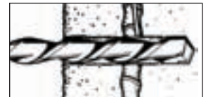
3. Return to hammer drilling to desired depth
