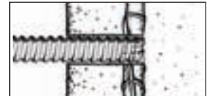
2. Using same size rebar cutter as masonry bit, rotary only through rebar
