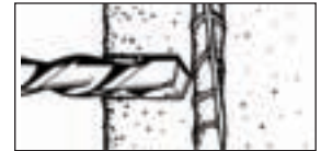
1. Stop hammer bit when rebar is encountered
