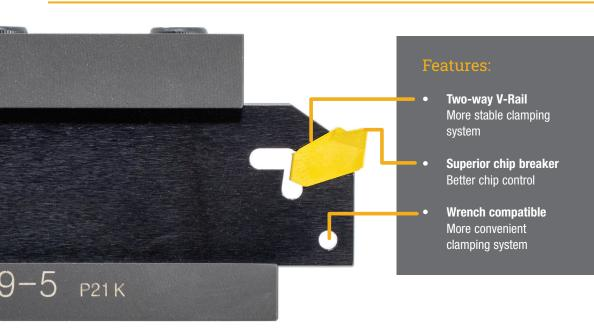
The stable clamping system of an insert and a holder is the most important factor in parting and deep grooving due to vibration from a long overhang, and narrow machining width causing unexpected fracture of the insert and breakage of the holder.
